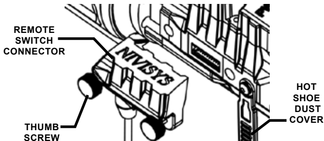
Figure 2-20 Remote Switch Installation
