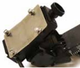
Quick Disconnect Attaches NVAG to visor / helmet.
