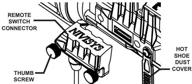
Figure 2-13 Remote Switch Installation
